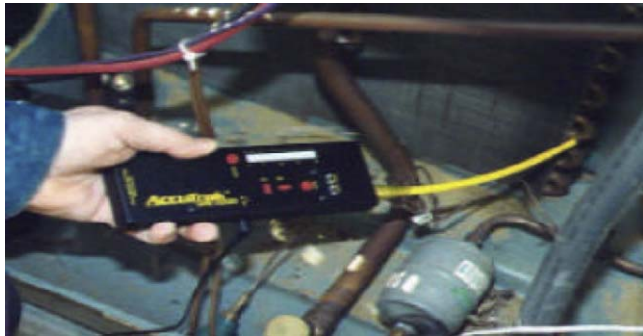
Fig. 24. Ultrasonic leak detection probe [35].
