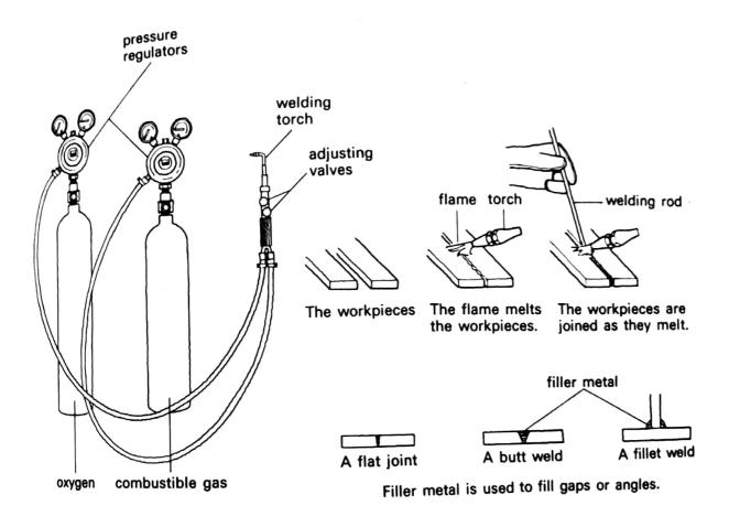
In gas welding, it is necessary to use a mixture of two gases. To create a hot enough flame, a combustible gas must be mixed with oxygen. Although acetylene (C<sub>2</sub>H<sub>2</sub>) is normally used, the combustible gas need not be acetylene. Hydrogen or petroleum gases (propane, for example) can also be used.
