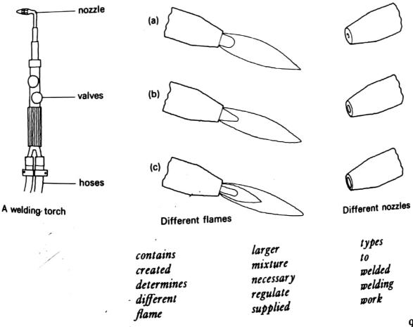
The welding gases are supplied . . . . the blowpipe through separate hoses. The blowpipe has two valves to . . . . the flow of each gas to the nozzle. In gas welding, three different . . . . of flame may be used:
