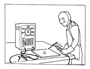
The earth clamp must be attached to the workpiece or (else) the current cannot flow.
