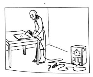
The earth clamp must be attached to the workpiece (in order) to complete the circuit.
