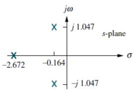
Stable system's closed-loop poles (not to scale)
