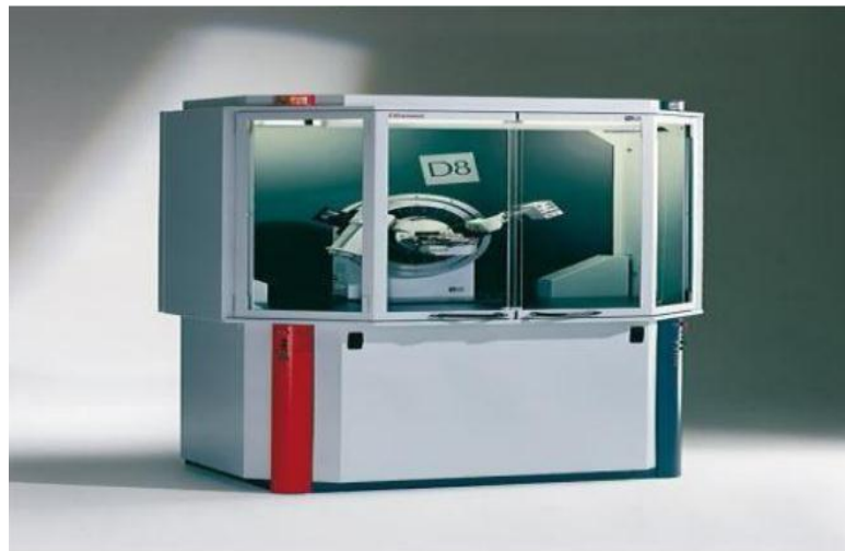
Figure 3.8. The image of Bruker AXS D8 Advanced type powder diffract meter
