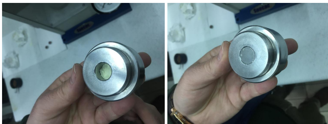
Figure 3.6. Pressing of the sample
