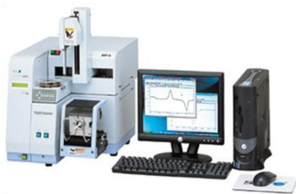
Figure 3.7. Image of the Perkin Elmer DTA/TG measurement system
