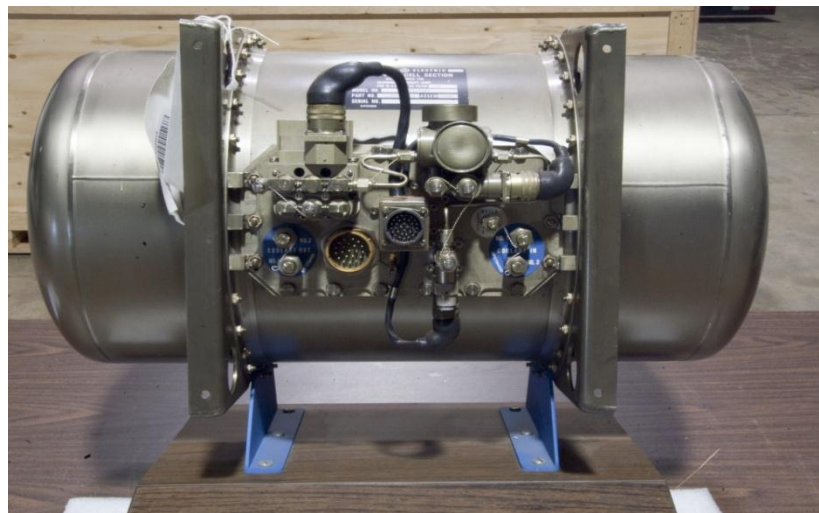
Figure 1.3. Proton exchange membrane (PEM) fuel used in Gemini spacecraft
