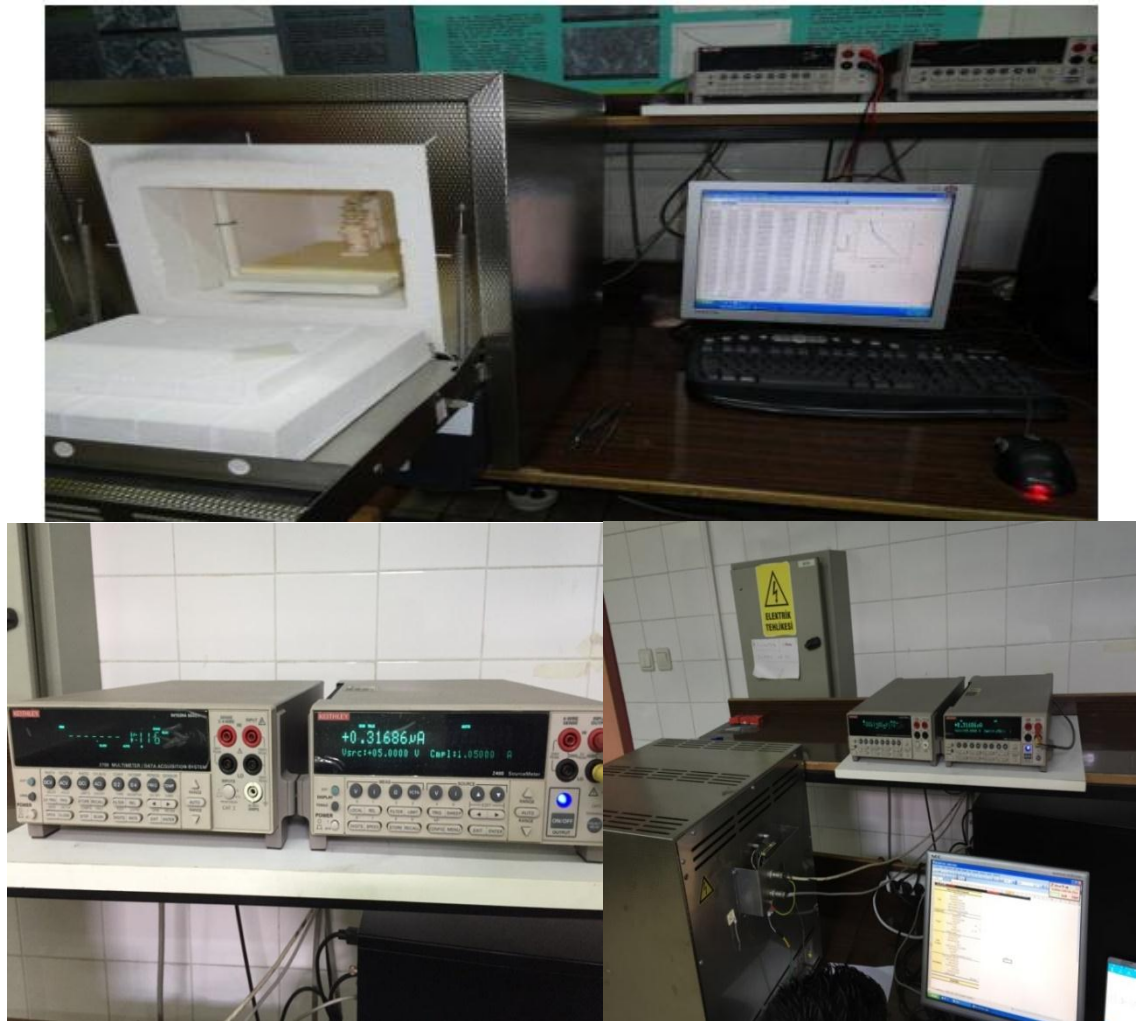
Figure 3.9. Computer controlled electrical conductivity measurement system
