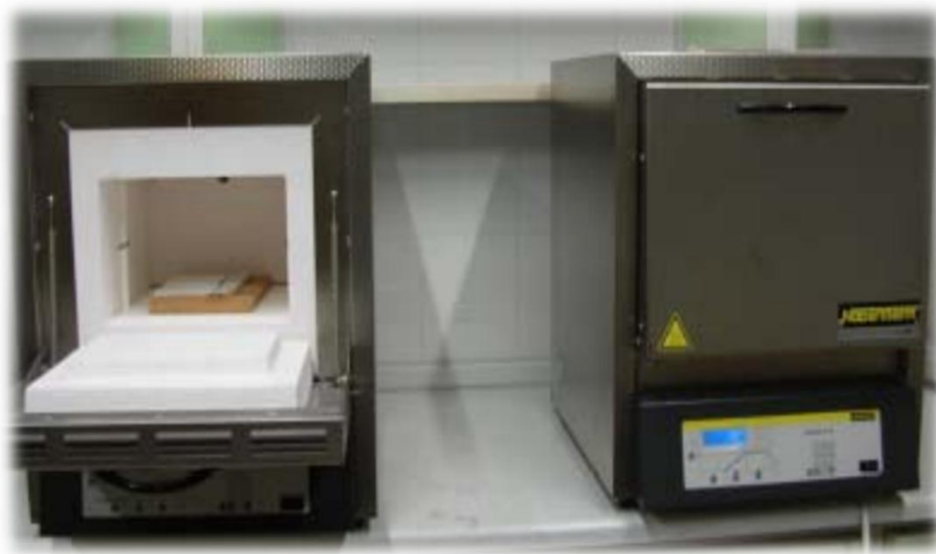
Figure 3.2. Furnaces used for solid state reactions
