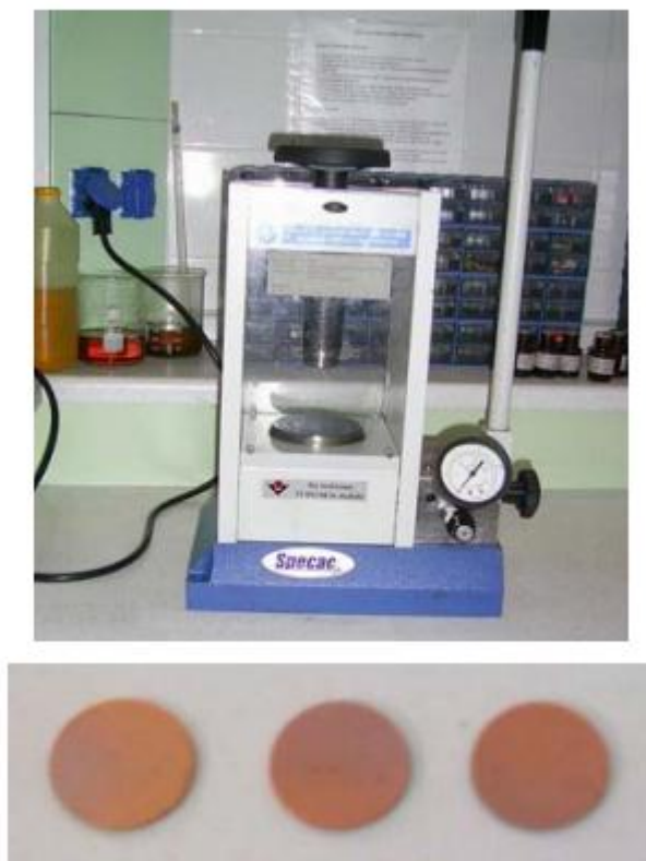
Figure 3.5. Manual hydraulic presses and some solid electrolyte materials sintered after packaging
