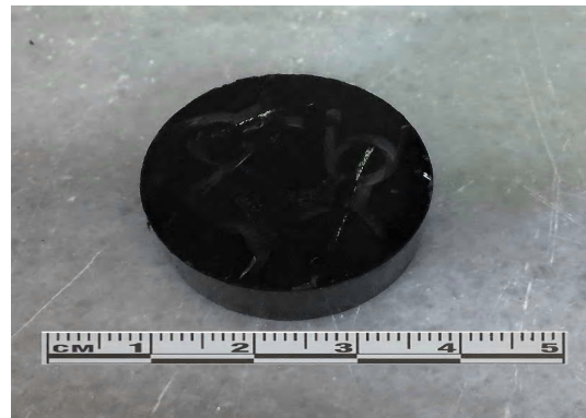
Figure 3.9. Hot mounting ribbon sample
