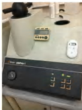
Figure 3.7. Struers Lapopress 1 device
