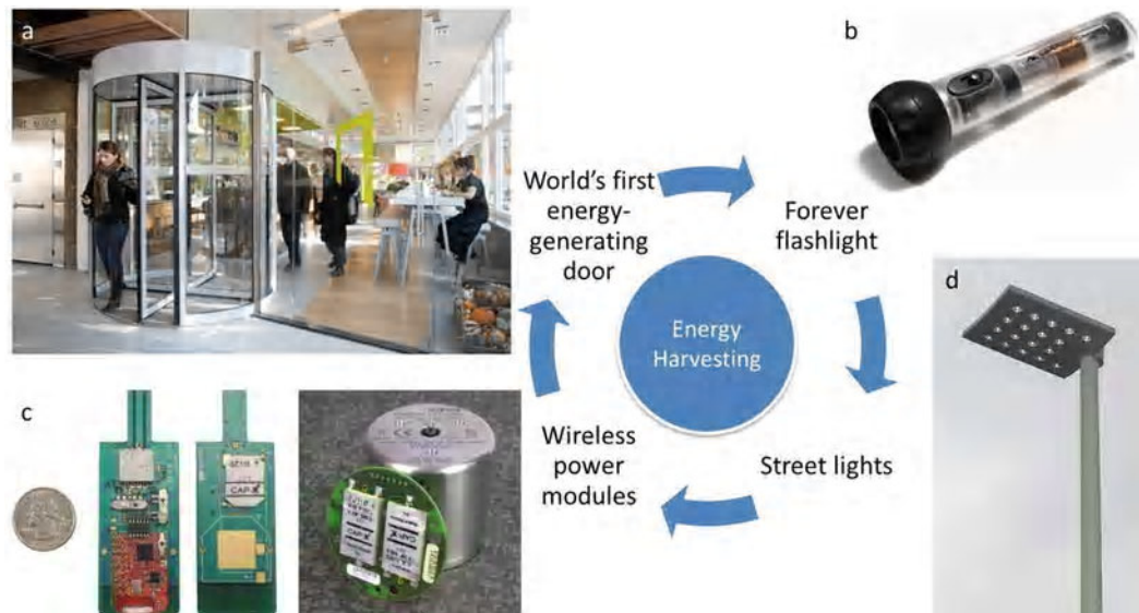
Figure 2.5 Typical applications of supercapacitors for energy harvesting a) World's first energy-generating revolving door, Netherlands, b) a mechanically powered flashlight, c) wireless power modules, and d) a stand-alone power source for a street light.
