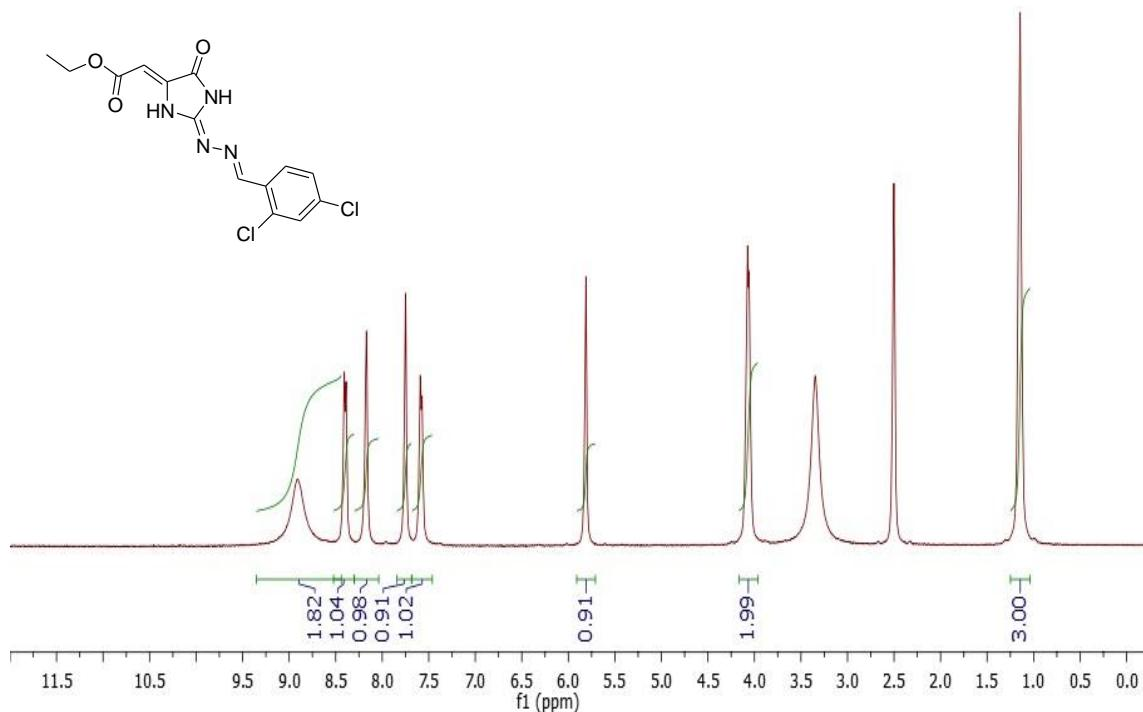
Figure 3.34.  $^1\text{H-NMR}$  spectrum of B4
