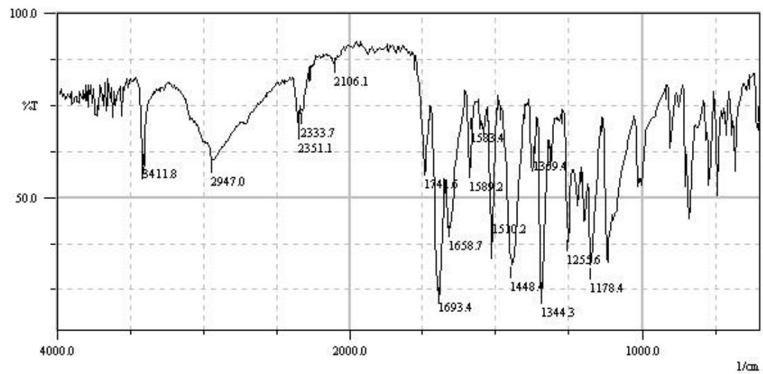
Figure 3.15. FT-IR spectrum of A5
