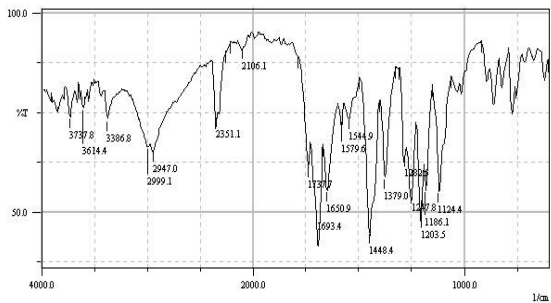
Figure 3.18. FT-IR spectrum of A6
