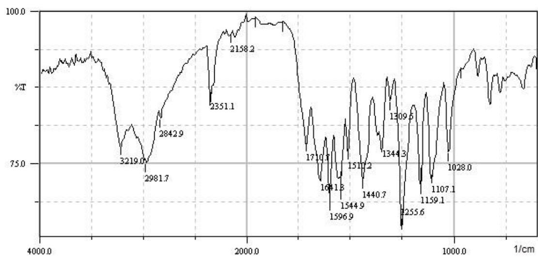
Figure 3.39. FT-IR spectrum of B5
