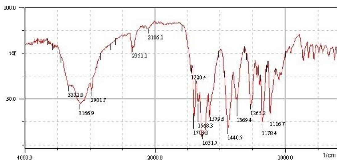
Figure 3.36. FT-IR spectrum of B4
