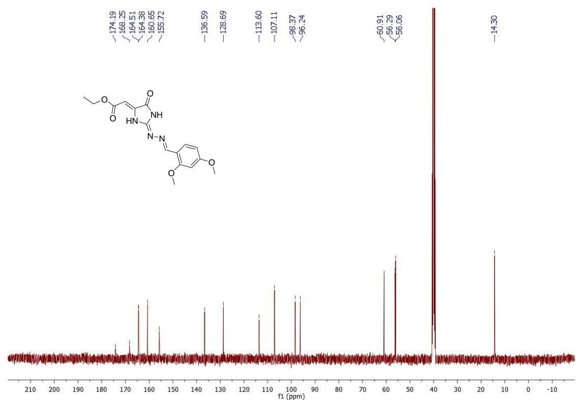
Figure 3.47.  $^{13}\text{C}$ -NMR spectrum of B8
