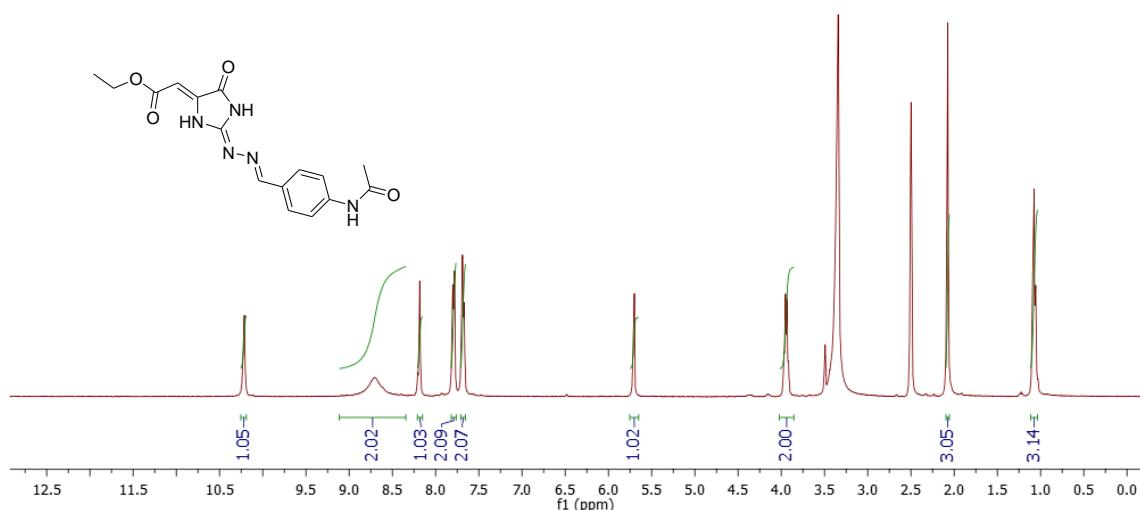
Figure 3.31.  $^1\text{H-NMR}$  spectrum of B3
