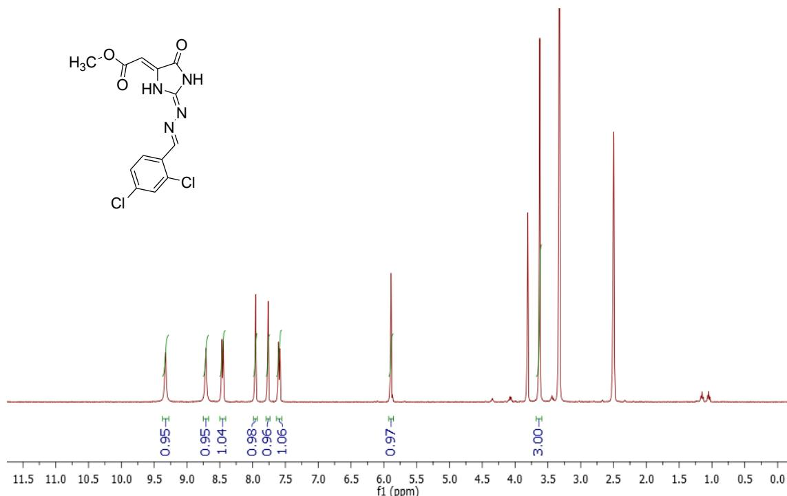
Figure 3.16. <sup>1</sup>H-NMR spectrum of A6
