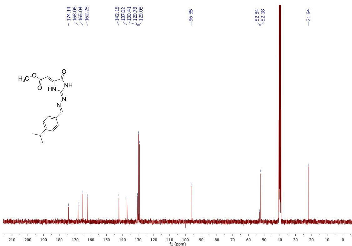
Figure 3.20.  $^{13}\text{C}$ -NMR spectrum of A7
