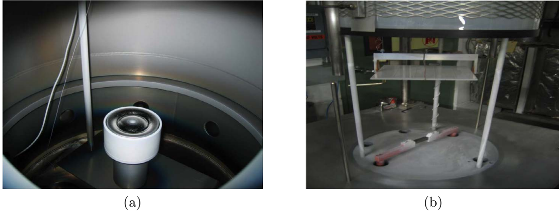
Figure 7.1: Para-Terphenyl (pTp) evaporation (a) and Anthracene (AN) sputtering (b) on quartz plates [94].
