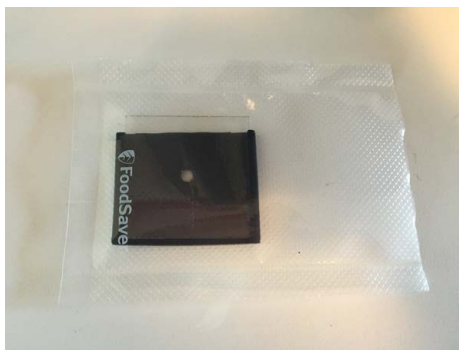
Figure 7.5: PEN sample before irradiation in a vacuum bag.
